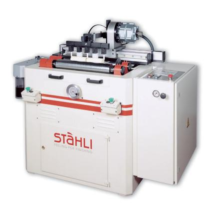
The CLM 150-1500 range of machines stands for time-saving centreless cylindrical lapping and polishing of longer work pieces between two parallel-running rollers.
