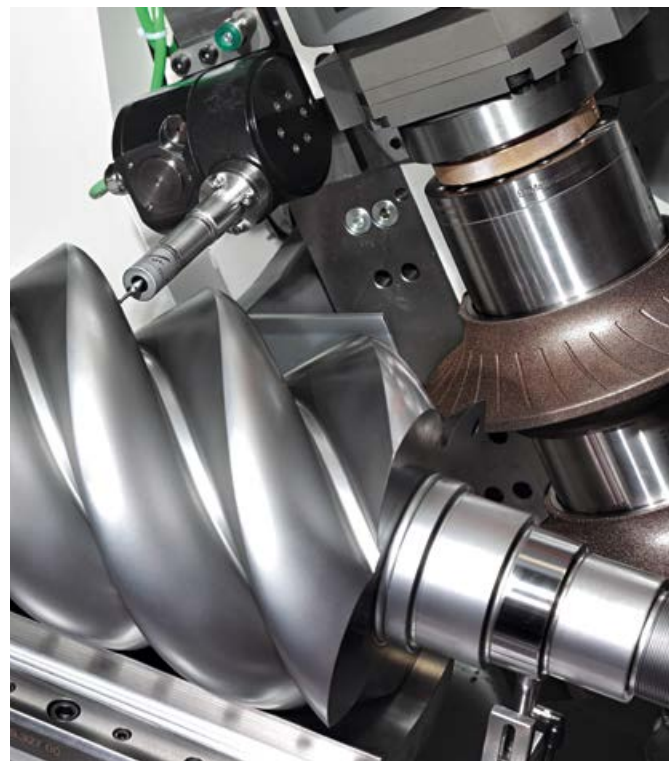
RX 120 with compact automation concept with integrated deburring station
