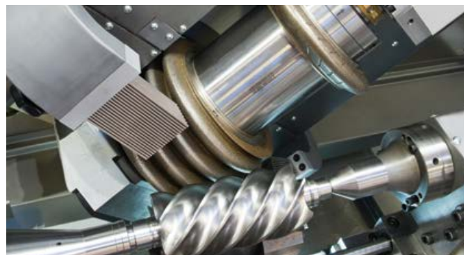
RX 120 with compact automation concept with integrated deburring station
