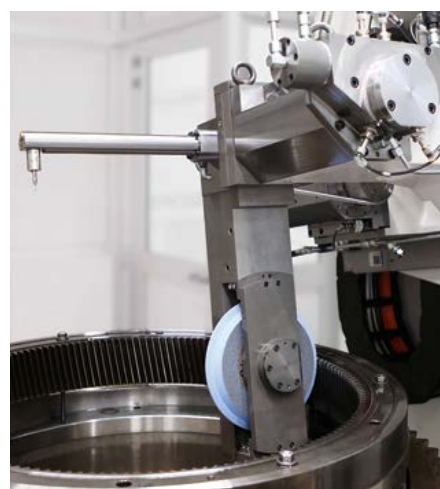
Special spindles (option) for the use of small grinding wheels
