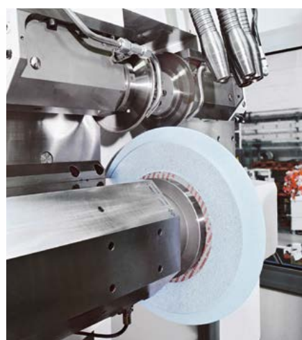
Special spindles (option) for the use of small grinding wheels
